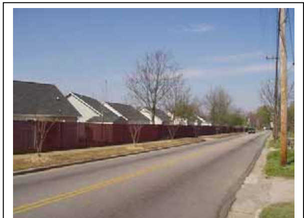
Reverse frontage conditions result when homes back up to a public street. This development pattern should be avoided where possible.
